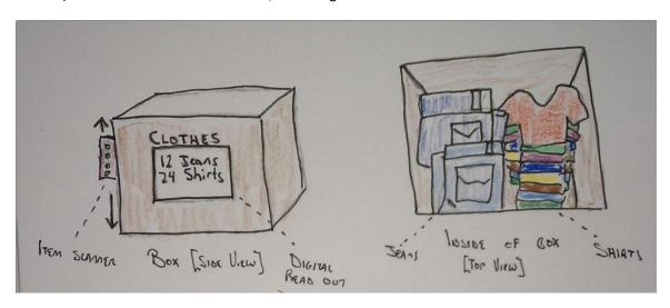
How this futuristic organizer works is that the scanner will scan the box every time an item goes in our out of the box. A computer system will calculate what items are in the box, how many of each, and how long each item has in the box. The digital read out will then state how many items are in the box.
